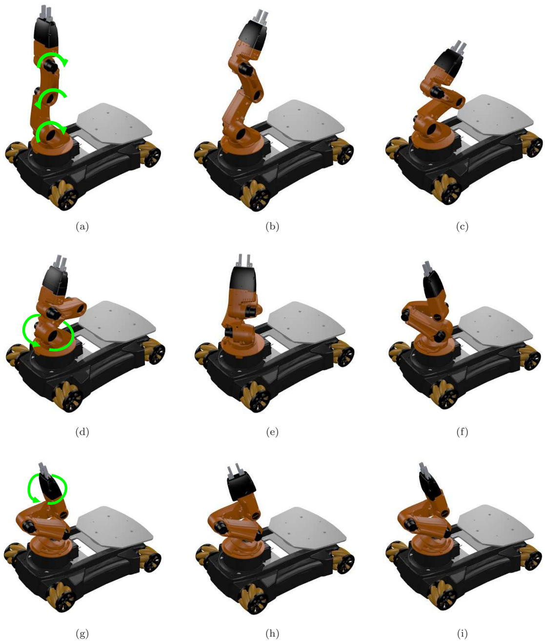
Figure 3.1: Procedure to move the manipulator into the home position: all joints are moved to their mechanical stops. Figures (a) to (c) show how to move the joints 2, 3 and 4 to the home position. Figures (d) to (f) illustrate how to rotate the first joint. Figures (g) to (i) show how to rotate the gripper.
